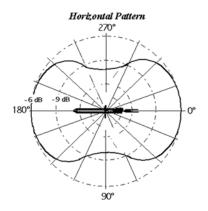
Fig. 8 Horizontal-Plane Radiation Pattern of the DL7PE-MicroVert
