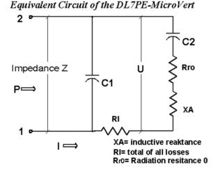
Fig. 3: Equivalent circuit including C1 ("dead" Capacity). X<sub>A</sub> stands for the reactance Coil, while R<sub>1</sub> is the summary of all losses.
