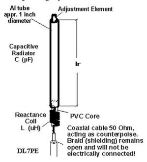
Principle design of the DL7PE-MicroVert
