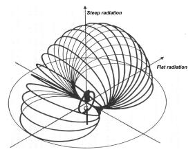
Fig. 7 Radiation pattern of a vertical small magnetic Loop more or less identical with that of the DL7PE-MicroVert
